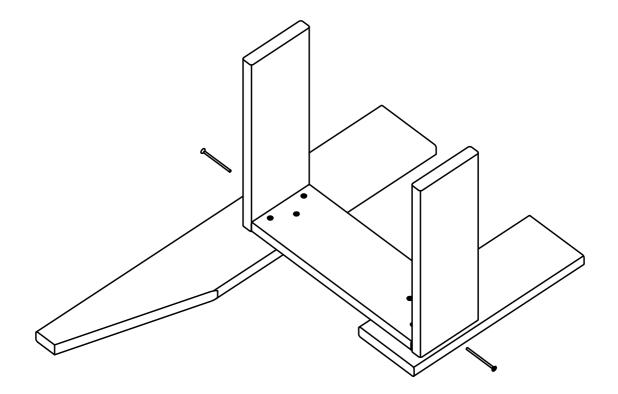
Pre-drill the boards. When driving a screw next to the edge of a board, it is good practice to pre-drill to avoid the wood spiltting.
