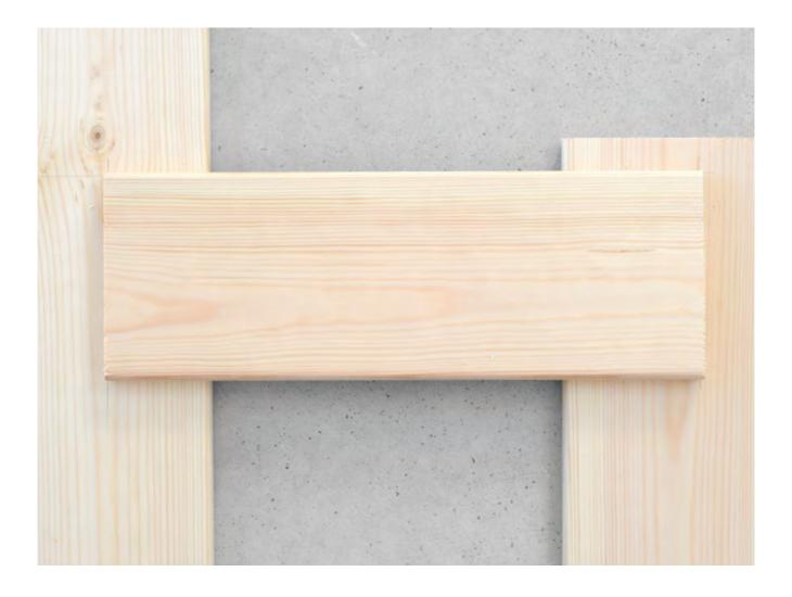
Pre-position before screwing (align bottom of the legs).
